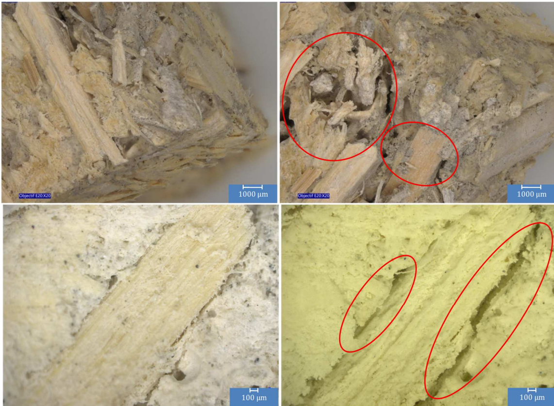
Fig. 6. Images of hemp concrete microstructure by Keyence microscope. On the left: before aging, on the right: after aging.
