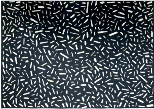
Fig. 2. Used hemp shives for particle size analysis.
