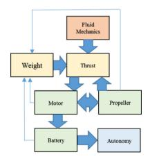
Figure 8. Simplified diagram of relations between the main components or parameters in the optimization of the flight time.
