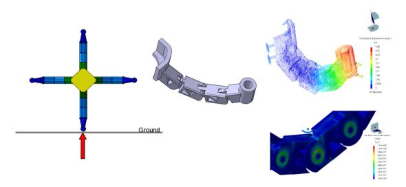
Figure 10. Optimization based on a critical case - fall of 2 m absorbed by only one leg.
