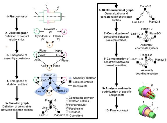
Figure 1. Design steps with the SKL-ACD approach.
