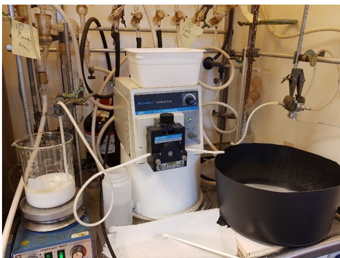
Figure 2. Picture of setup used for producing Al(OH)fumarate spheres by spraying the MOF/alginate slurry (to the left) through a nozzle (to the right) by use of a peristaltic pump (middle).
