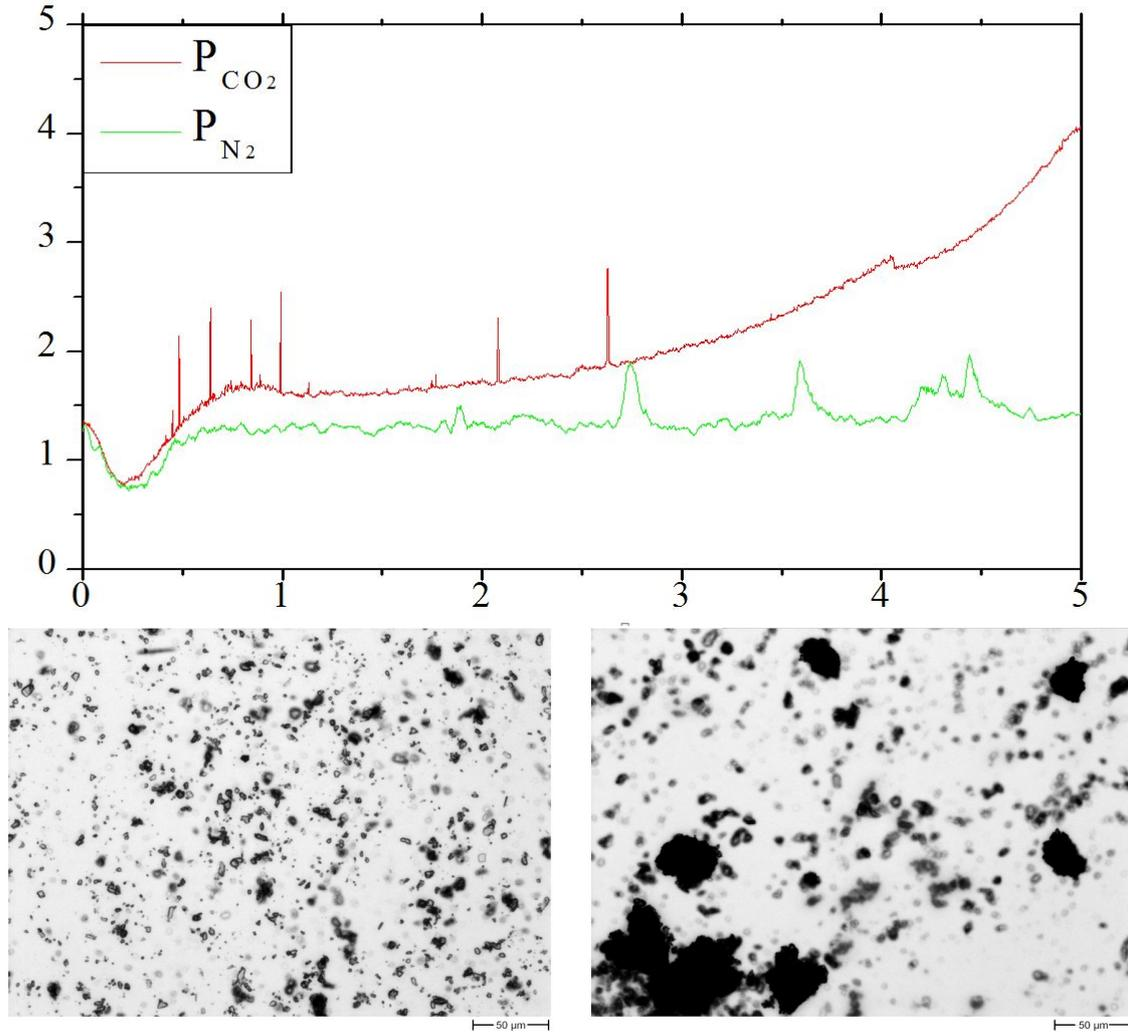
FIG. 5: Comparison of the apparent viscosity recorded under pressure of nitrogen or carbon dioxide (top), and snapshots of the resulting suspensions (bottom), obtained for tests at volume fraction  $\phi = 20\%$ ,  $\dot{\gamma} = 100 \text{ s}^{-1}$ ,  $T = 100 \text{ }^\circ\text{C}$ , and  $P_{N_2} = 40 \text{ bars}$  (left) and  $P_{CO_2} = 40 \text{ bars}$  (right), respectively.
