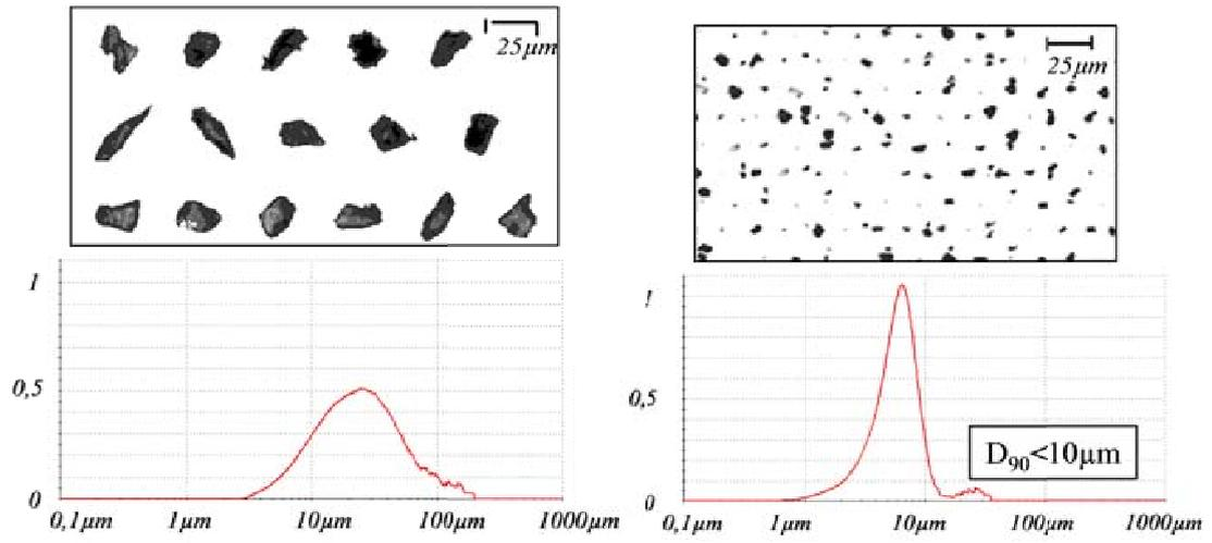
FIG. 1: Size distribution and snapshots of the olivine particles, before (left) and after (right) micronization.
