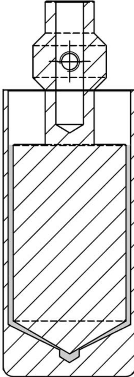
FIG. 2: Geometry of the rheometer cell. The conical bottom of the cell ensures an almost homogeneous shear rate in the whole volume of sheared suspension.
