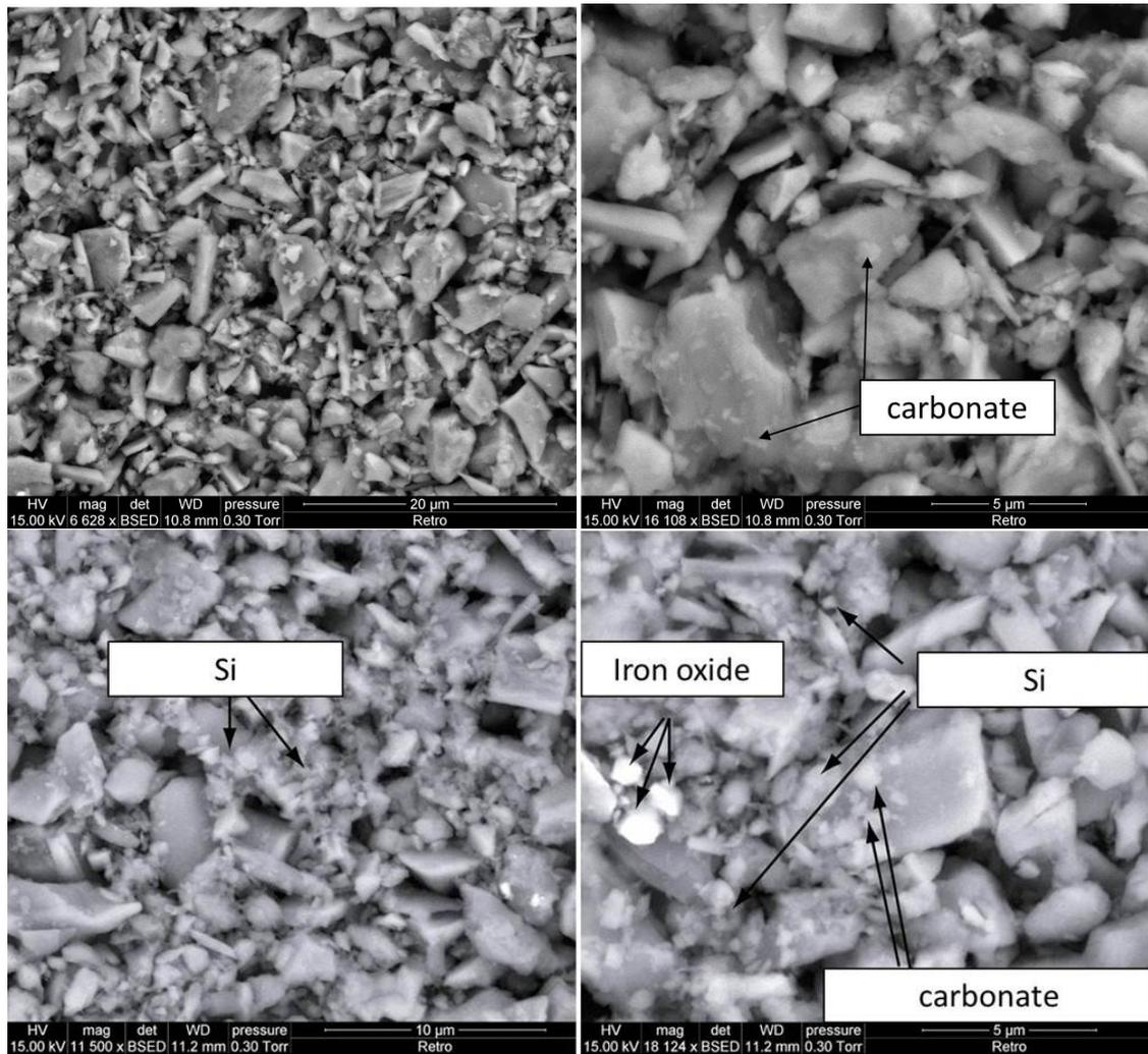
FIG. 6: Scanning Electron Microscope (SEM) images of the particles after 7 hours (top) and 13 hours (bottom) for a slurry at volume fraction  $\phi = 20\%$ , sheared at  $\dot{\gamma} = 100 \text{ s}^{-1}$ , at  $T = 80 \text{ }^\circ\text{C}$ , and  $P_{\text{CO}_2} = 40 \text{ bars}$ .
