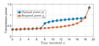
Fig. 2: We plot the optimal power  $p_n^*$  minimizing  $J_{TT}(p, n)$ , and the required power  $\underline{p}_n$  for given values of n.
