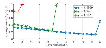
Fig. 3: Average power consumed  $J_{\mathrm{TT}}(p_n^*, n)$  using the optimal transmission power  $p_n^*$  for the given n and  $\mu$ .
