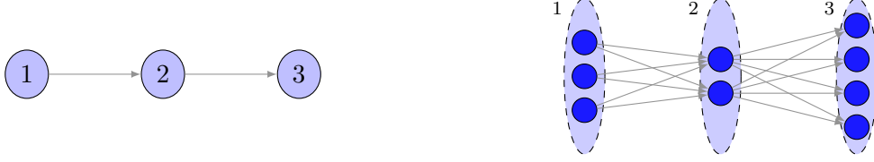
Figure 2: A sequence of customers in the auxiliary network for the ATSP and its generalization to delivery options in the GVRPTW. There are three, two and, four options per delivery request in this example, i.e., |O_1^N| = 3 , |O_2^N| = 2 , and |O_3^N| = 4 .
