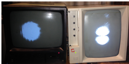
Figure 2: Output of the cavity for the vertical and horizontal polarizations, injected to different TEM cavity modes and monitored with two cameras.
