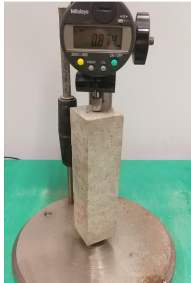
Figure 5 – Measuring axial expansion with the extensometer.
