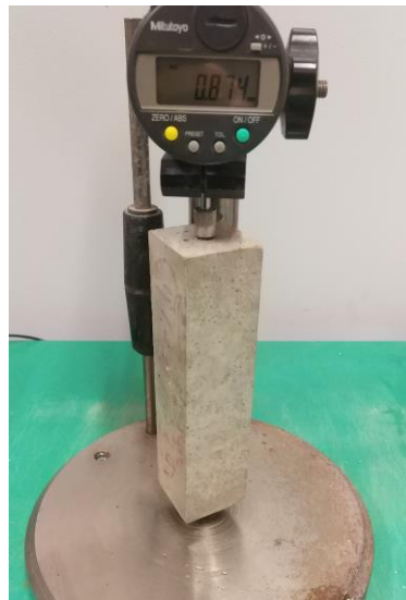
Figure 5 – Measuring axial expansion with the extensometer.
