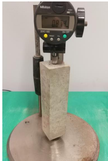
Figure 5 – Measuring axial expansion with the extensometer.
