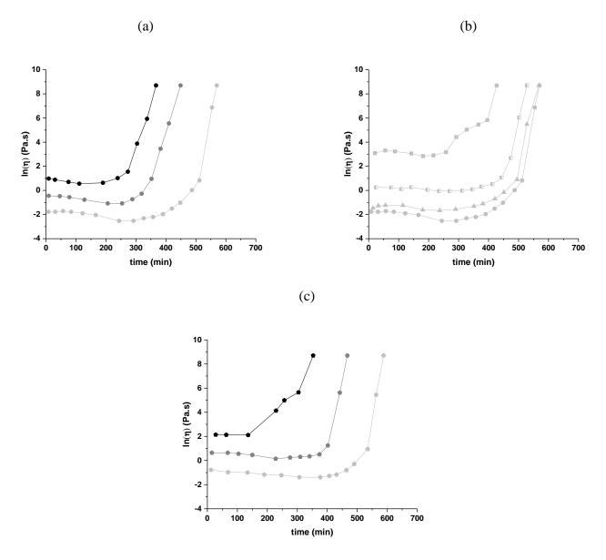
Figure 5. Viscosity  $\eta$  (± 1%) as a function of time (± 30 min) for  ${}^{a}M_{x}W_{y}G_{z}$  samples: (a)  ${}^{a}M_{100}$ (a = (•) 0.6, (•) 0.8 and (•) 1), (b) (•)  ${}^{0.6}M_{70}W_{30}$ , (•)  ${}^{0.6}M_{45}W_{55}$ , (▲)  ${}^{0.6}M_{90}G_{10}$  and (c) (•)  ${}^{0.6}M_{78}W_{18}G_{4}$ , (•)  ${}^{0.8}M_{85}W_{11}G_{4}$  (•)  ${}^{1}M_{87}W_{10}G_{3}$ .
