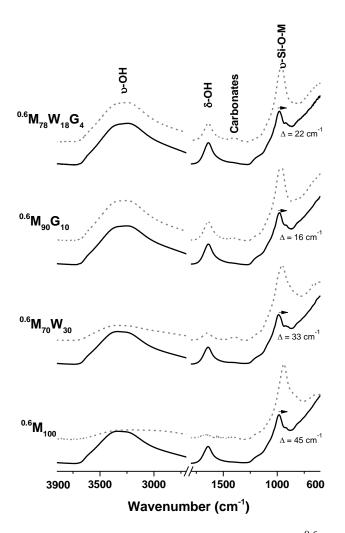
Figure 2. FTIR spectra obtained at — t = 0 and at 700 min for the <sup>0.6</sup>M<sub>100</sub>, <sup>0.6</sup>M<sub>70</sub>W<sub>30</sub>, <sup>0.6</sup>M<sub>90</sub>G<sub>10</sub> and <sup>0.6</sup>M<sub>78</sub>W<sub>18</sub>G<sub>4</sub> samples.
