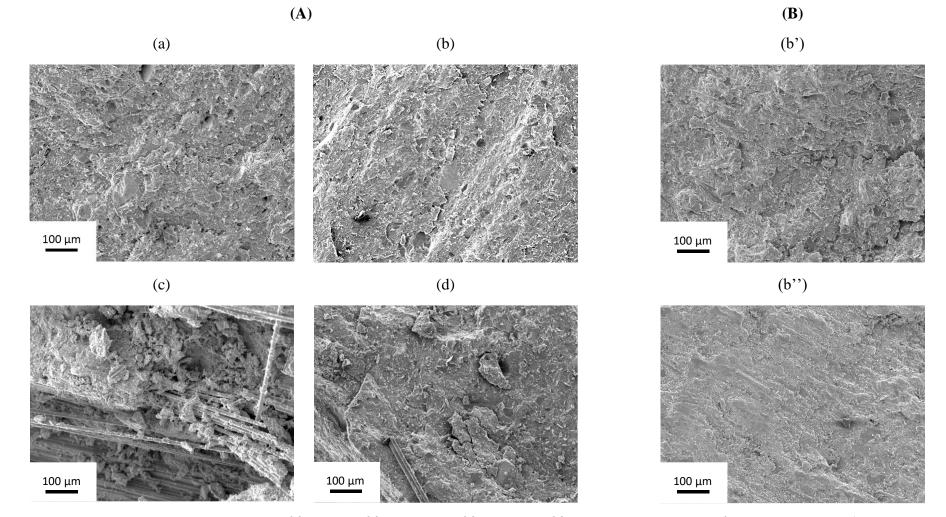
Figure 8. SEM micrographs of the (A) (a)  ${}^{0.8}M_{100}$ , (b)  ${}^{0.8}M_{74}W_{26}$ , (c)  ${}^{0.8}M_{92}G_8$ , (d)  ${}^{0.8}M_{85}W_{11}G_4$ , and (B) (b')  ${}^{0.6}M_{70}W_{30}$  and (b'')  ${}^{1}M_{78}W_{22}$  various formulations.
