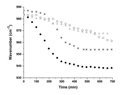
Figure 3. Si-O-M band wavenumber  $(\pm 4 \text{ cm}^{-1})$  as a function of time for  $\bullet$  <sup>0.6</sup>M<sub>100</sub>,  $\blacksquare$  <sup>0.6</sup>M<sub>70</sub>W<sub>30</sub>,  $\blacktriangle$  <sup>0.6</sup>M<sub>90</sub>G<sub>10</sub> and  $\bigcirc$  <sup>0.6</sup>M<sub>78</sub>W<sub>18</sub>G<sub>4</sub> samples.
