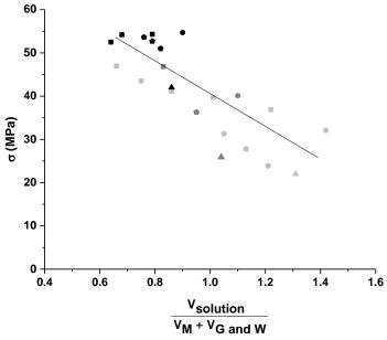
Figure 9. Evolution of (a) the weight loss (± 2 %) and (b) the compressive strength (± 3 MPa) as function of the *ratio*  $\frac{V_{solution}}{V_M + V_{G \text{ and } W}}$  for the (•)  ${}^aM_x$ , (•)  ${}^aM_xW_y$ , (•)  ${}^aM_xG_z$  and (•)  ${}^aM_xW_yG_z$  geopolymer composites, with a = • 0.6, • 0.8 and • 1 (see Table 2).
