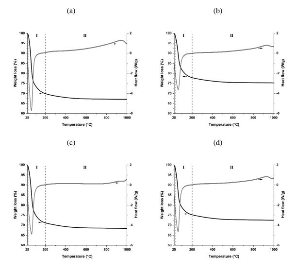
Figure 4. Thermal analysis curves (DTA-TGA) as functions of the temperature for the (a)  ${}^{0.6}M_{100}$ , (b)  ${}^{0.6}M_{70}W_{30}$ , (c)  ${}^{0.6}M_{90}G_{10}$  and (d)  ${}^{0.6}M_{78}W_{18}G_4$  samples.
