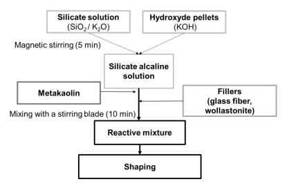
Figure 1. Protocol used to synthesize geopolymer composites.
