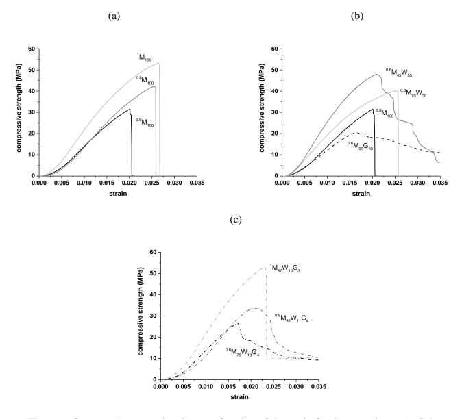
Figure 6. Compressive strength value as a function of the strain for the geopolymer (a)  ${}^{a}M_{100}$  binders and (b)  ${}^{0.6}M_xW_y$ ,  ${}^{0.6}M_xG_z$  and (c)  ${}^{a}M_xW_yG_z$ , geopolymer composites.
