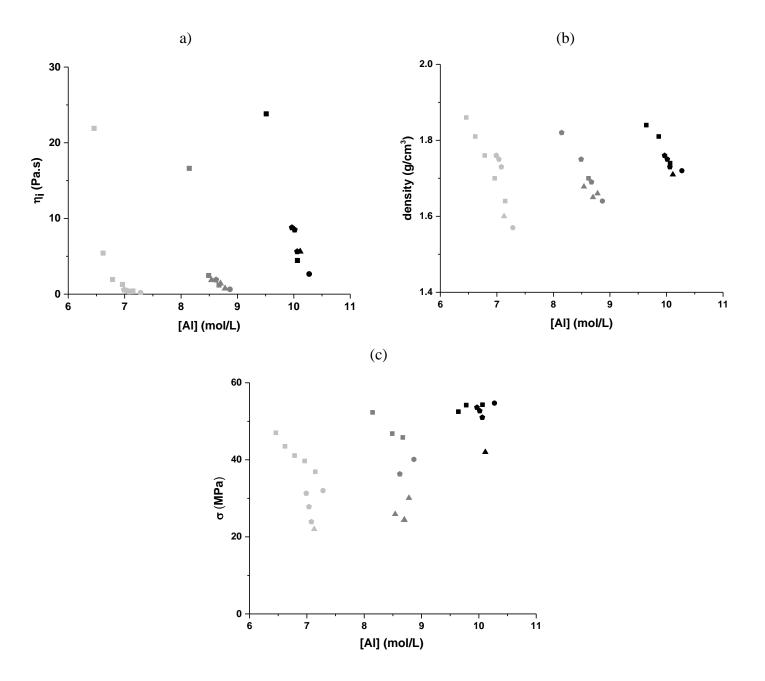
Figure 7. Evolution of (a) the initial viscosity  $\eta i (\pm 1\%)$ , (b) the density  $(\pm 1 \text{ g/cm}^3)$  and (c) the compressive strength  $\sigma (\pm 3 \text{ MPa})$  as functions of the aluminum concentration [A1] for the ( $\bullet$ )  ${}^{a}M_{x}$ , ( $\blacksquare$ )  ${}^{a}M_{x}W_{y}$ , ( $\blacktriangle$ )  ${}^{a}M_{x}G_{z}$  and ( $\bullet$ )  ${}^{a}M_{x}W_{y}G_{z}$  geopolymer composites, with  $a = \bullet 0.6$ ,  $\bullet 0.8$  and  $\bullet 1$  (see Table 2).
