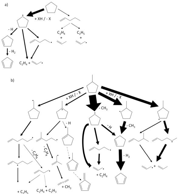
Figure 9: Reaction pathway analysis of the oxidation of a) cyclopentane and b) methylcyclopentane in a JSR at T = 1150 K, p = 1 atm,  $\tau = 0.07$ s, and  $\varphi = 1$  (the size of the arrows is proportional to the flow rate).
