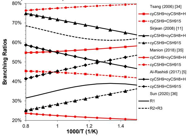
Figure 3: Comparison of the branching ratio between ring opening  $cyC5H9 \Rightarrow C5H915$  (R1) and hydrogen atom elimination (R2). R3 is the prompt dissociation of pent-1-en-5-yl.
