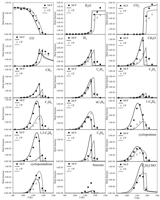
Figure 6: Experimental and computed mole fraction profiles obtained from the oxidation of cyclopentane (empty triangles-dashed line) and methylcyclopentane (filled circles-full line) in a JSR at  $\varphi = 0.5$ , p = 1 atm,  $\tau = 0.07$ s.
