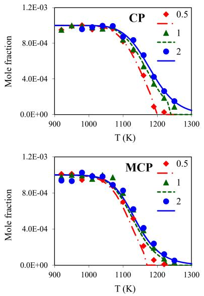
Figure 5: Experimental (symbols) and computed (lines) mole fraction profiles obtained from the oxidation of cyclopentane (CP) and methylcyclopentane (MCP) in a JSR at p = 1 atm,  $\tau = 0.07$ s, and  $\phi = 0.5$  (red),  $\phi = 1$  (green), and  $\phi = 2$  (blue).
