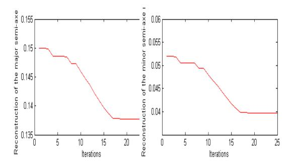
Fig. 6. Reconstruction of the semi-major axe  $r_2$  and the semi-minor axe  $r_{22}$  of the internal ellipse  $\Omega_2$  using the Newton method
