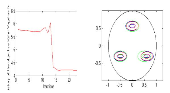
Fig. 7. The history of the energy gap cost functional and reconstruction of three coated ellipses(the intial shape(green), the approximated shape(blue), the exact shape(red))
