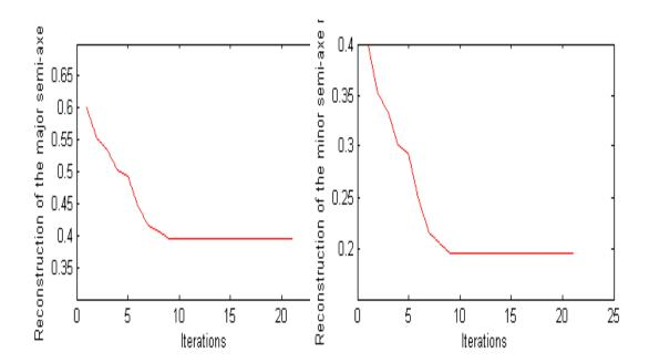
**Fig. 2.** Reconstruction of the semi-major axe  $r_1$  and the semi-minor axe  $r_{11}$  of the external ellipse  $\Omega_1$  using the Newton method.
