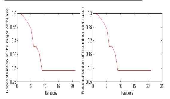
Fig. 3. Reconstruction of the semi-major axe  $r_2$  and the semi-minor axe  $r_{22}$  of the internal ellipse  $\Omega_2$  using the Newton method
