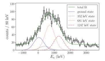
FIG. 11. Excitation energy spectrum for <sup>95</sup>Sr. The total  $\gamma$ -ray yield has been used to constrain the area of Gaussian peaks and the excitation energy spectrum has been fitted with four components and a constant background. The component representing the 352 keV state has been fixed to the upper limit obtained from the  $\gamma$ -ray analysis.
