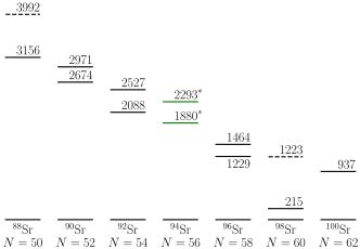
FIG. 15. Energy systematics of the  $0^+$  states in even-mass Sr isotopes. Levels drawn with dashed lines are tentative assignments [17,28–33]. The newly observed  $0^+$  states <sup>94</sup>Sr from the present experiment are marked with an asterisk.
