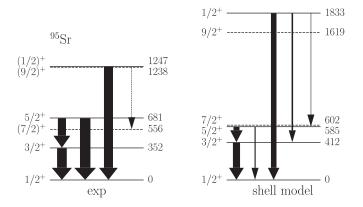
FIG. 16. Proposed level scheme of  ${}^{95}$ Sr. The left side shows the experimental levels with energies in keV and the spin and parity assignments from this work. The widths of the arrows are proportional to the relative intensity of the observed  $\gamma$ -ray transition. Dashed levels and transitions have not been observed in the present work. The right side shows the result of shell-model calculations. Here the widths of the arrows indicate the branching ratios.
