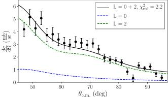
FIG. 12. Angular distribution of tritons gated on both the ground and 618 keV states in <sup>95</sup>Sr. The data are compared to DWBA reaction model calculations assuming removal of a neutron from the  $3s_{1/2}$ orbital with L = 0 for the ground state (blue) and from the  $2d_{5/2}$ orbital with L = 2 for the 681 keV state (green). The combination of L = 0 and L = 2 best fitting the data is shown by the solid black line.
