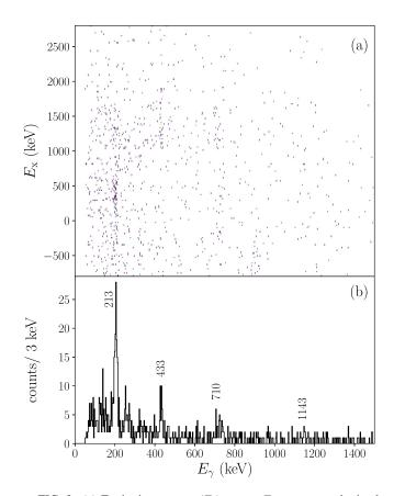
FIG. 3. (a) Excitation energy  $(E_x)$  versus  $E_{\gamma}$  spectrum obtained from the <sup>2</sup>H(<sup>94</sup>Sr, t) reaction. (b) corresponds to the  $\gamma$ -ray energy spectrum.
