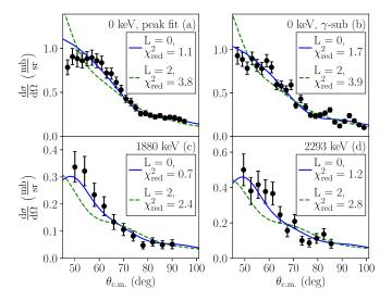
FIG. 7. Angular distribution of tritons for L = 0 transfer reactions to final states in <sup>94</sup>Sr. (a) and (b) show the results of the two methods to extract the ground-state distribution. The newly discovered 0<sup>+</sup> states are shown in (c) and (d). The L = 0 and L = 2 DWBA calculations are fitted to the data, and are shown by the blue (solid) and green (dashed) lines and labeled with their respective reduced  $\chi^2$  values.
