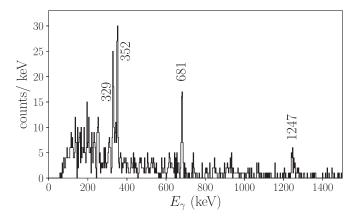
FIG. 10.  $\gamma$ -ray energy spectrum for the <sup>2</sup>H(<sup>96</sup>Sr, t) <sup>95</sup>Sr reaction. A gate on excitation energies below 1800 keV has been applied.
