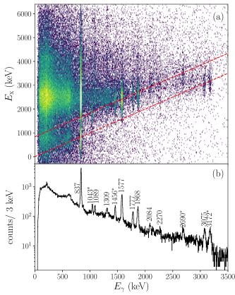
FIG. 5. (a) Excitation energy  $(E_x)$  versus  $E_{\gamma}$  spectrum for <sup>94</sup>Sr populated via the <sup>2</sup>H(<sup>95</sup>Sr, *t*) reaction. The dashed lines indicate the location of direct ground-state decays and decays to the first excited 2<sup>+</sup> state at 837 keV. (b) corresponds to the  $\gamma$ -ray spectrum. The newly observed transitions are marked with asterisks.
