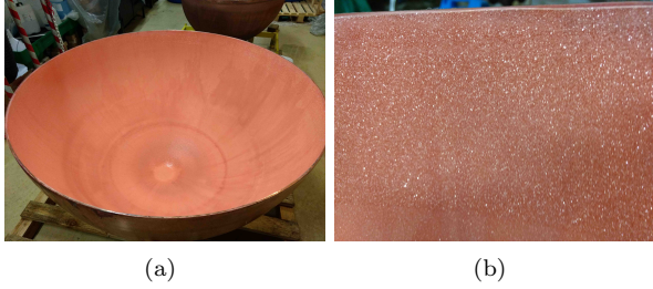
Figure 10: (a) The inner surface of the second hemisphere after electroplating and (b) a close-up of the surface.
