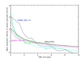
**Fig. 16.** Mean expansion velocity of the parent granules leading to the development of the largest TFGs. The dashed line corresponds to the expansion velocity dR/dt, where R(t) is the radius of the disk area such that  $\pi \times R^2(t) = A(t) = a + b \times t$ , where *a* and *b* are constants, fitted to the simulation.
