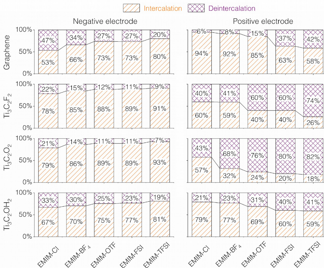
Figure 8: Proportions of intercalation and deintercalation at the maximum charged state for all the electrode materials and electrolytes studied in this work.
