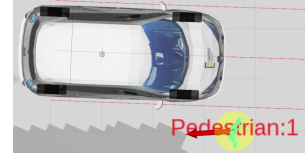
Fig. 4. Perceived pedestrian and its estimated orientation.
