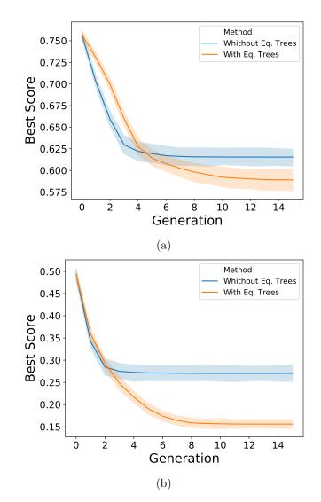
Fig. 2: Fitness value of the best random forest individual over iterations on synthetic (a) and fall detection datasets (b).
