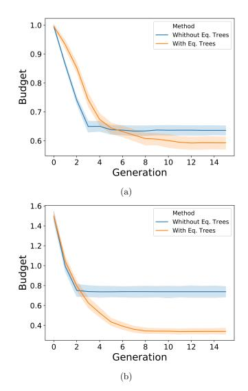
Fig. 3: Mean prediction time cost of the best random forest individual over iterations on synthetic (a) and fall detection datasets (b).
