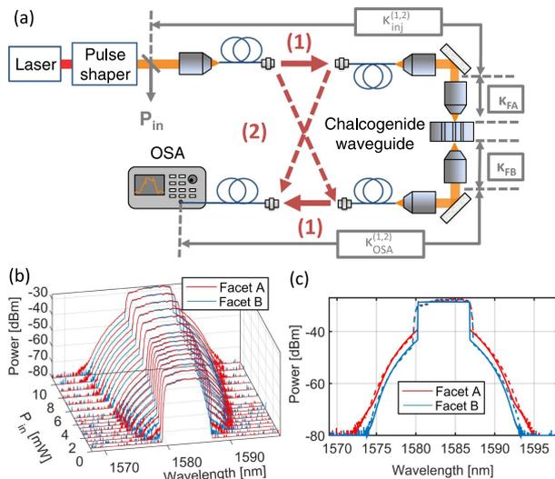
**Fig. 2.** (a) Bidirectional nonlinear transmission setup. Following the injection from both chalcogenide facets A and B, (b) measured output spectra varying the average input powers  $P_{in}$  between 0.5 and 11 mW, and (c) experimental (solid lines) and simulated (dashed lines) output spectra at  $P_{in} = 11$  mW, where the nonlinear phase shift for the simulated spectra coincides to  $\phi_{NL}^{(A)} = 0.59$  rad and  $\phi_{NL}^{(B)} = 0.39$  rad.
