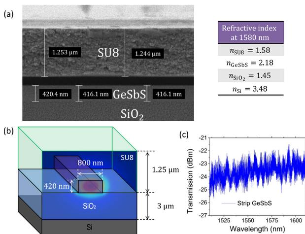
**Fig. 1.** (a) SEM image and refractive indices at 1580 nm of the layer stack. (b) GeSbS waveguide structure with a superposition of the fundamental TE-mode profile. (c) Linear optical transmission of the 1 cm long chalcogenide waveguide.
