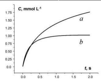
Figure 10. Evolution of surface concentration of 2, formed at the limiting current potential through the mechanisms (1, 3 - 5) (a) and (1, 7 - 9) (b) under the conditions of chronoamperometry.
