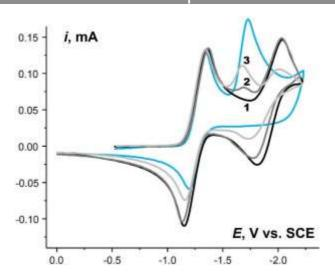
**Figure 5**. Cyclic voltammograms of **1** (7 mmol L<sup>-1</sup>) in DMF/0.1 M Bu<sub>4</sub>NClO<sub>4</sub> in the presence of 0 (*1*), 3.5 (2) and 10.0 (3) mmol L<sup>-1</sup> LiClO<sub>4</sub>. Blue curve: **1** (7 mmol L<sup>-1</sup>) in DMF/0.1 M LiClO<sub>4</sub>. Scan rate v = 0.1 V s<sup>-1</sup>.
