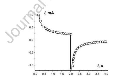
**Figure 4**. CA curves of **1** (20 mmol  $L^{-1}$ ) in DMF/0.1 M Bu<sub>4</sub>NClO<sub>4</sub> at the limiting current potentials: experimental (line) and simulated (circles).
