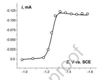
**Figure 3**. Experimental CA currents (2 s after applying the potential pulse) of **1** (10 mmol  $L^{-1}$ ) in DMF/0.1M Bu<sub>4</sub>NClO<sub>4</sub> solution (circles) and the simulated curve (line).
