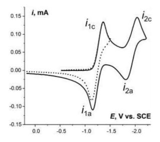
**Figure 1.** Cyclic voltammograms of **1** (7 mmol  $L^{-1}$ ) in DMF/0.1 M Bu<sub>4</sub>NClO<sub>4</sub> at the potential scan rate of 0.1 V s<sup>-1</sup>.
