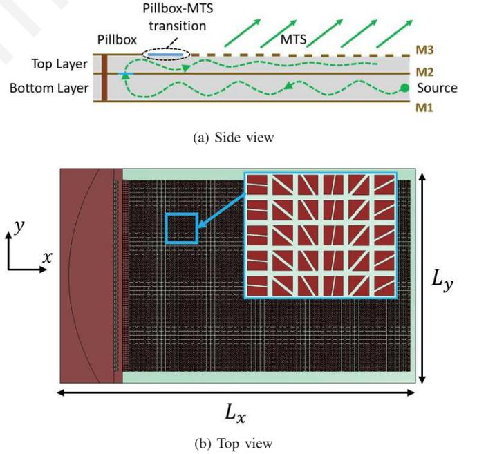
Fig. 3. Final antenna configuration. The two-layer structure is represented in (a), while the modulated MTS and the pillbox top layer are shown in (b). The dimensions of the antenna are  $L_x = 17\lambda_0$  and  $L_y = 10.4\lambda_0$ , where  $\lambda_0$  is the free-space wavelength for  $f = 20.7\text{GHz}$ .
