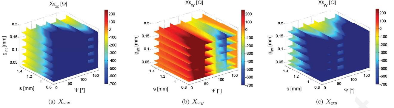
Fig. 2. 3-dimensional database relating the impedance components of (1) with the geometry of the patch in Fig. 1, where  $g_{int}$  is the internal gap size,  $s$  is the patch size and  $\Psi$  is the gap rotation.
