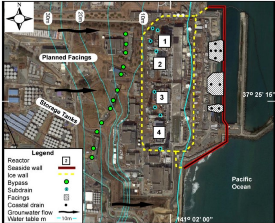
Fig. 2. Plan view of storage facilities and engineering works to contain radioactively contaminated groundwater.
