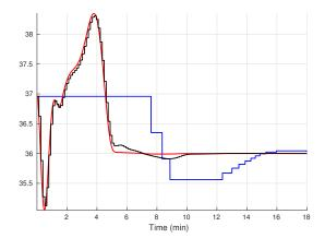
Fig. 1. Time-evolution of the velocity control input: the continuous-time control U (27) (depicted in red line), the event-triggered boundary control  $U_d$  (30),(32) (static triggering condition with time regularization T=0.13) (depicted in black line) and the event-triggered boundary control  $U_d$  (30),(33) (dynamic triggering condition) (depicted in blue line).
