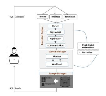
Figure 5 – Internal Architecture of Hyrise
