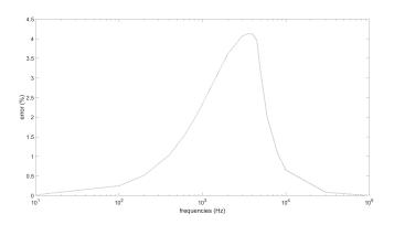
Figure 11: Influence of a periodic input perturbation  $v_{in}(t) = v_{inc} + v_{invar} sin(2\pi ft)$ . A traditional control law is used, improved by adaptive techniques. The maximal amplitude error on the output voltage is plotted against the frequency of the perturbation.
