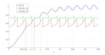
Figure 1: The signal  $x(\tau)$  is plotted in blue and the signal  $\tilde{x}_T(t,\tau)$  is plotted for  $t = t_1$  in red and for  $t = t_2$  in green, versus its second time scale  $\tau$ .
