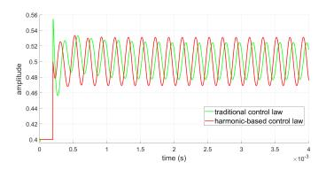
Figure 14: Output regulation with a periodic input perturbation of critical frequency f = 5kHz. The resulting duty-cycle commands are plotted for traditional (temporal) control in green and harmonic-based control in red.
