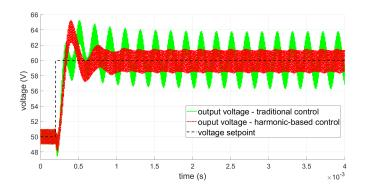
Figure 12: Output regulation with a periodic input perturbation of critical frequency f = 5kHz. The resulting output voltages are plotted for traditional (temporal) control in green and harmonic-based control in red.
