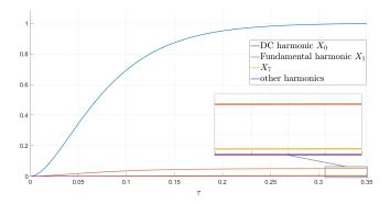
Figure 2: The generalized Fourier coefficients  $X_k(\tau)$  of signal  $x(\tau)$  (blue signal in Figure 1) are plotted against time. The periodic steady state is clearly defined by constant harmonics.
