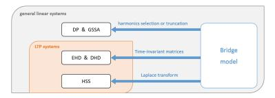
Figure 5: Links between the bridge model unifying the different harmonic modeling approaches. All harmonic models can be derived from the state space of the bridge model in Proposition 4.
