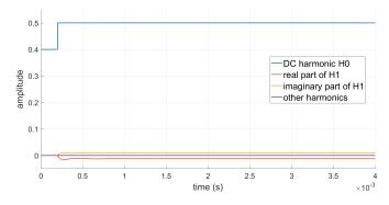
Figure 15: Output regulation with a periodic input perturbation rejection by harmonic-based control. The resulting command law harmonics are plotted.
