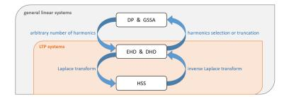
Figure 4: Links between the different harmonic modeling approaches.
