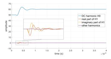
Figure 13: Output regulation with a periodic input perturbation rejection by harmonic-based control. The resulting output voltage harmonics are plotted.
