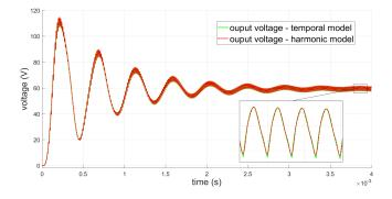
Figure 9: Comparison of the output voltage from temporal model and harmonic model in the exponential basis of frequency f = 25kHz and with 12 harmonics.
