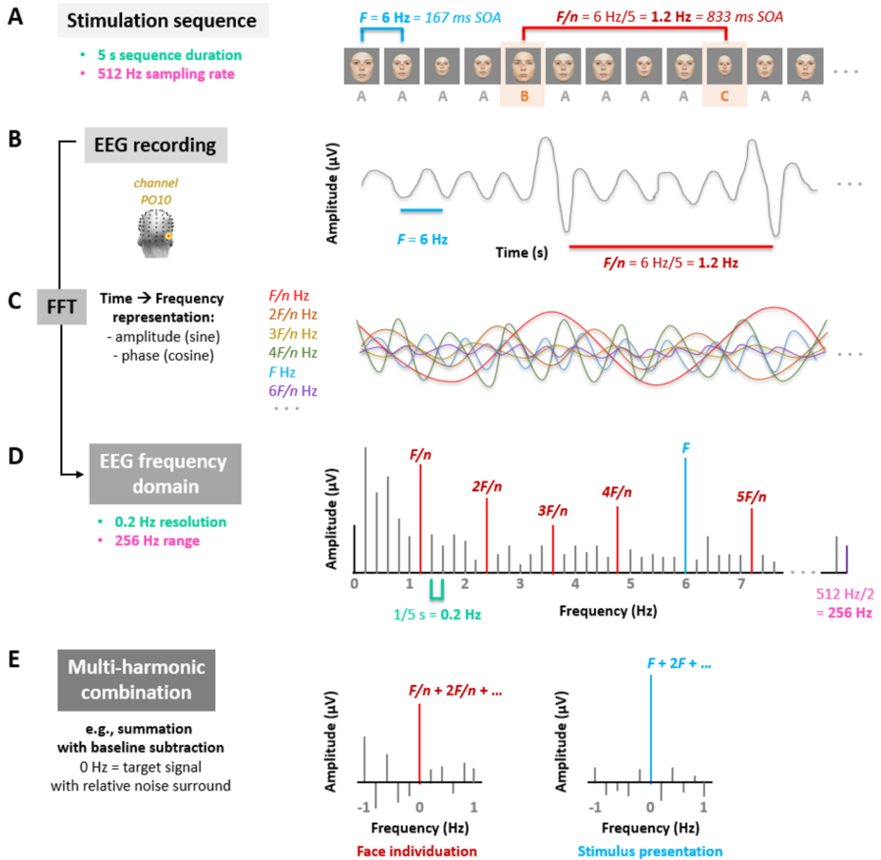
Figure 3. Basics of time to frequency domain representations for oddball FPVS with EEG.
