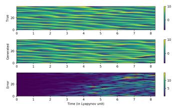
Fig. 8: The true L96 sequence (top), the sequence generated by the model trained on noisy data with r = 19.4% (middle) and the error between the true and the generated sequence (bot).
