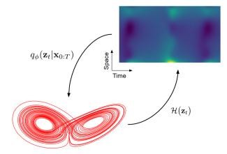
Fig. 10: Higher-dimensional Legendre observations governed by lower-dimensional L63 dynamics. Following [51], the observations (top right) are in a 128-dimensional space, while L63 dynamics (bottom left) are in a 3-dimensional space. The observation operator involves a non-linear mapping according to Legendre polynomials [51].
