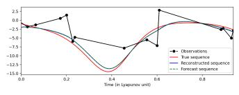
Fig. 6: An example of the the first dimension of the L63 system reconstructed by the inference module of DAODEN\_determ. The observations are noisy (r = 33%) and irregularly sampled with a missing rate of 87.5%.
