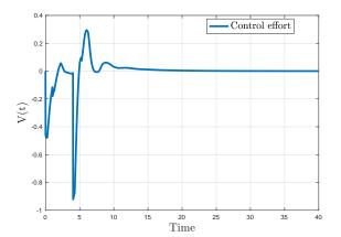
Fig. 3. Evolution of the control input V in closed-loop.
