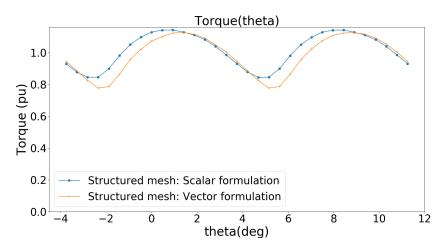
Figure 9: Torque with structured mesh
