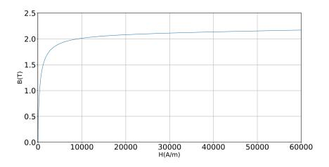
Figure 4: B-H curve of steel
