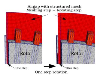
Figure 8: Structured mesh in airgap
