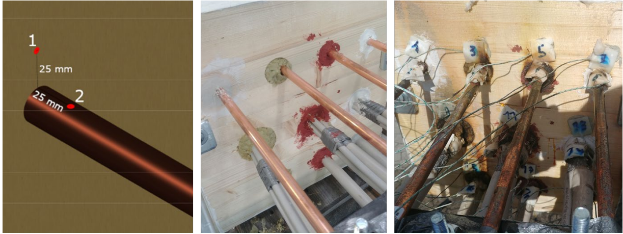
Fig. 8 Measure points (left), exemplary test assembly (middle), assembly after the test (right)
