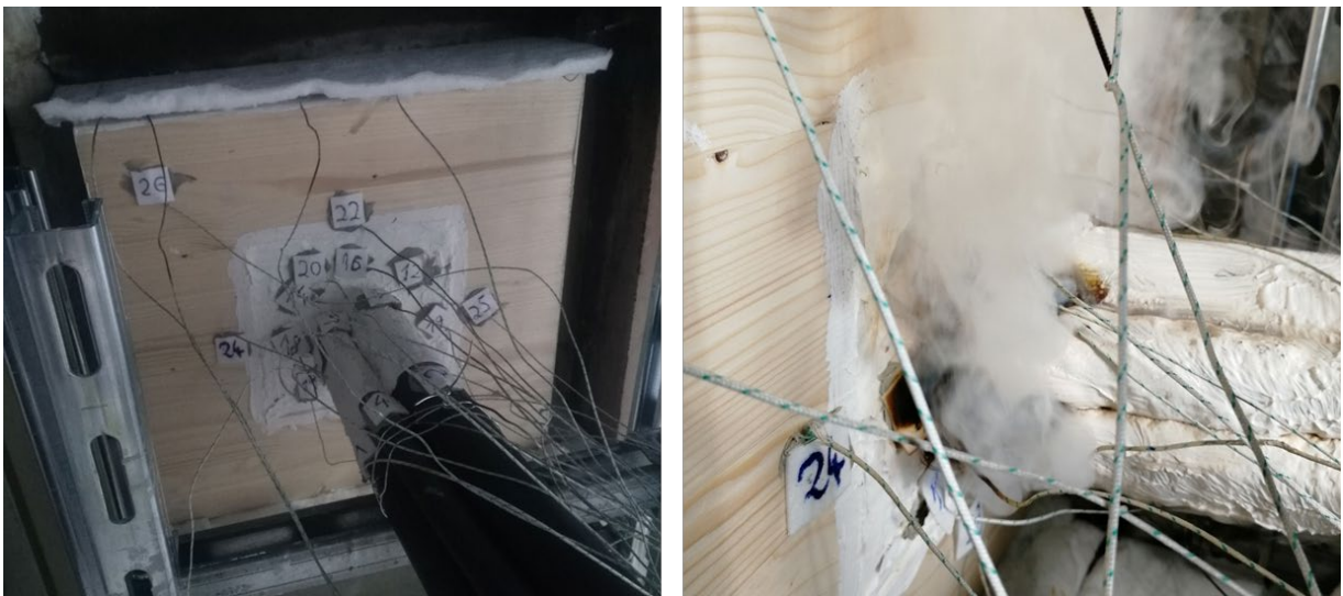
Fig. 3 Coated mineral wool slab with cables (service option “M” according to Annex A EN 1366-3 ) before the test and after 90 mins of exposure
