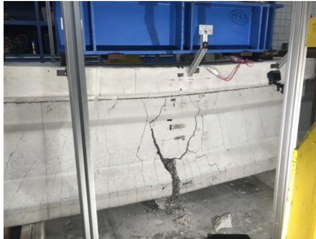
Fig. 5 Girder 4 at failure load (rupture of strands failure)
