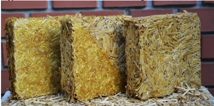
Fig. 1 Laboratory prototypes of the straw insulation
