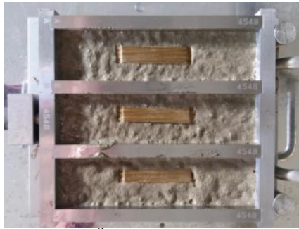
Fig. 1 A mould for three 40x40x160 mm 3 specimens – a demonstration of the steel fibres placement.
