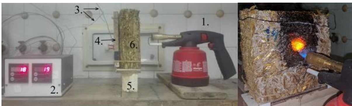
Fig. 5 Components of the experimental set-up used for measure fire resistance (left): 1.: gas lamp, 2.: digital thermometer, 3.: thermocouples, 4.: thermocouples fixing plate, 5.: specimen fixing stand, 6.: straw specimen. The specimen during the test (right)
