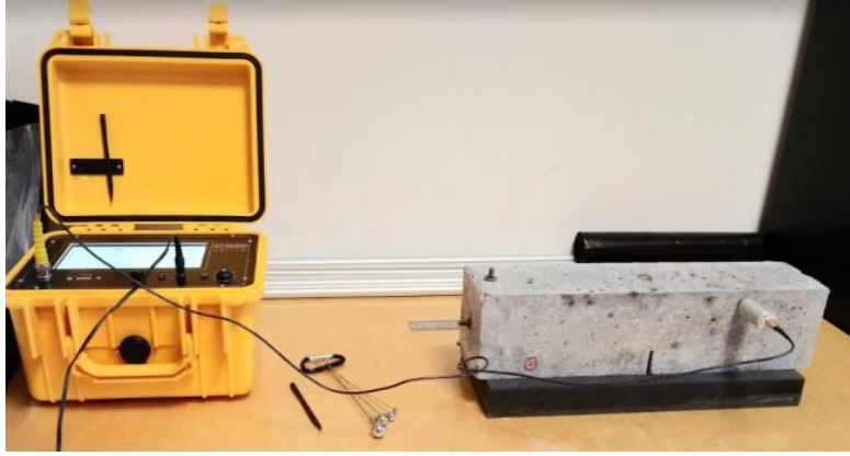
Fig.1 Stand for resonance frequency measurement of concrete prism samples.
