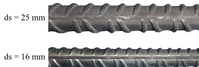
Fig. 1 Steel bars used in the tests
