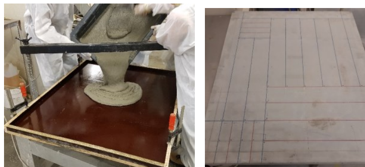
Fig. 3 Casting of the thin slab (left) and the layout of the plates sawn (right)
