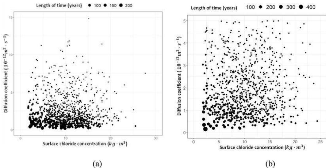
Fig. 2. Bivariate plot of (a) effective diffusion coefficient  $D_e$  ( $10^{-12} \text{ m}^2 \cdot \text{s}^{-1}$ ) as function of surface chloride concentration  $C_s$  ( $\text{kg} \cdot \text{m}^{-3}$ ) over 1000 simulated points, with (b) a zoom on interval ranges  $D_e$  in  $[0;5]$  ( $10^{-12} \text{ m}^2 \cdot \text{s}^{-1}$ ) and  $C_s$  in  $[0;25]$  ( $\text{kg} \cdot \text{m}^{-3}$ ) over 883 simulated points.
