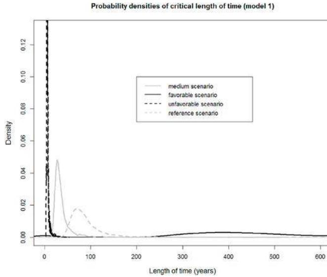
**Fig. 5.** Pdf of the critical length of time (year) to corrosion initiation for 4 scenarios: unfavorable (with  $D_e = 6.0 \times 10^{-12} \text{ m}^2 \cdot \text{s}^{-1}$ ), medium (with  $D_e = 0.66 \times 10^{-12} \text{ m}^2 \cdot \text{s}^{-1}$ ), reference (with  $D_e = 0.25 \times 10^{-12} \text{ m}^2 \cdot \text{s}^{-1}$ ) and favorable (with  $D_e = 0.1 \times 10^{-12} \text{ m}^2 \cdot \text{s}^{-1}$ ).
