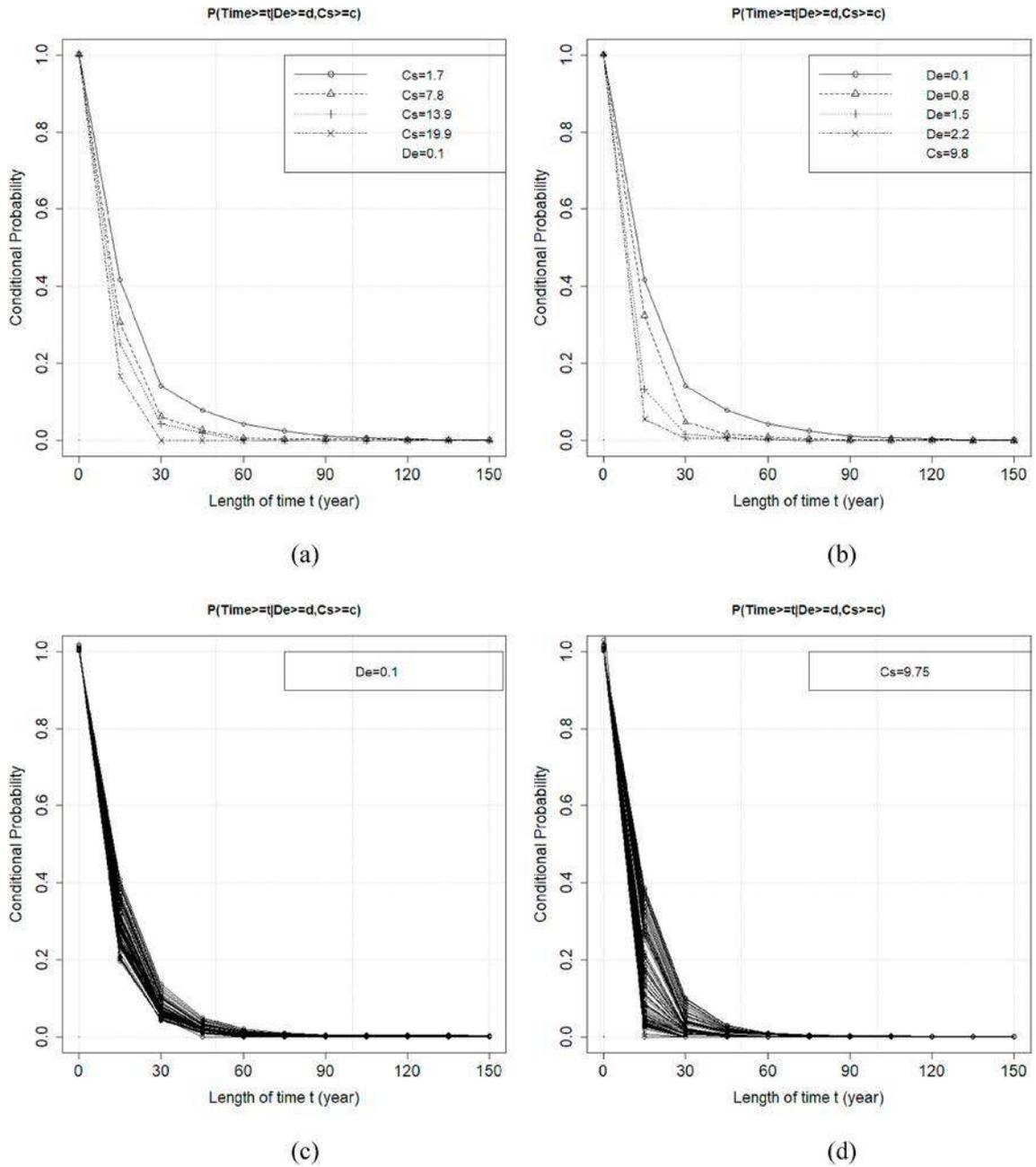
**Fig. 4.** Conditional probabilities of the critical length of time  $t$  (year) to corrosion initiation given the co-occurrence of effective diffusion coefficient  $D_e = 0.1 \times 10^{-12} \text{ m}^2 \cdot \text{s}^{-1}$  and (a) four and (c) one hundred values of surface chloride concentration ( $C_s, \text{ kg} \cdot \text{m}^{-3}$ ), and given the co-occurrence of  $C_s = 9.75 \text{ kg} \cdot \text{m}^{-3}$  and (b) four and (d) one hundred values of  $D_e$ .
