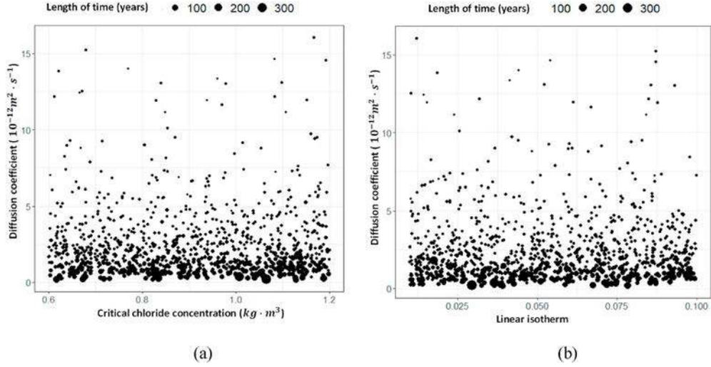
**Fig. 3.** Bivariate plot of effective diffusion coefficient ( $10^{-12} \text{ m}^2 \cdot \text{s}^{-1}$ ) as function of (a) critical chloride content ( $\text{kg} \cdot \text{m}^{-3}$ ) and (b) linear isotherm over 1000 simulated points.
