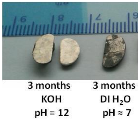
Figure 3: Shape, color and roughness change of 3 months aged Gd_6Co_{1.67}Si_3 material in KOH pH \geq 12 (left), in DI H_2O pH \approx 7 (right) .
