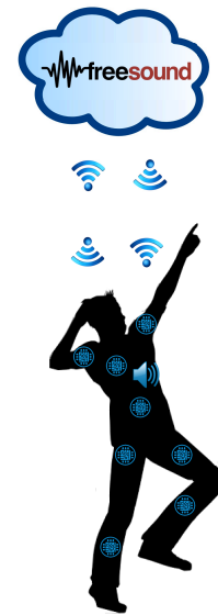
Fig. 4. A schematic representation of the sensor- and actuator-equipped garment presented in [19], which interacts with the audio content repository Freesound.org
