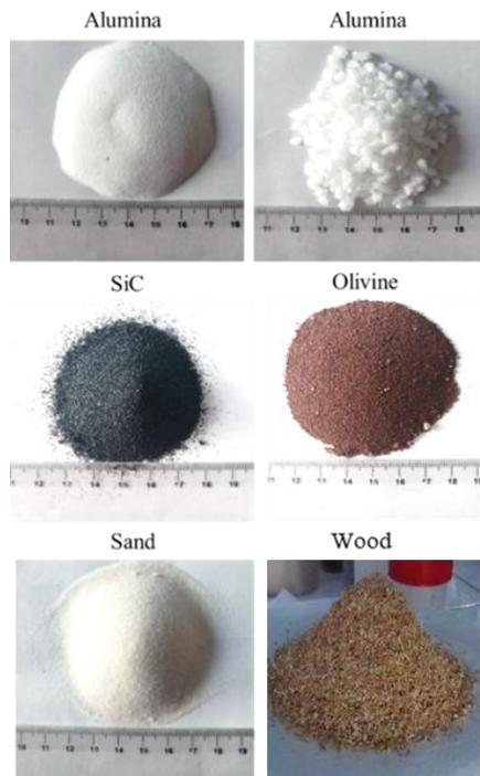
**Figure 2.** Studied inert bed and wood biomass particles
