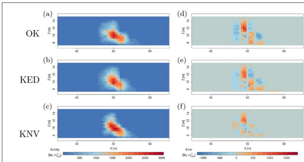
Fig. 2. Map of estimation obtained with the OK (a), KED (b) and KNV (c) approaches; and maps of corresponding estimation errors (d, e and f).
