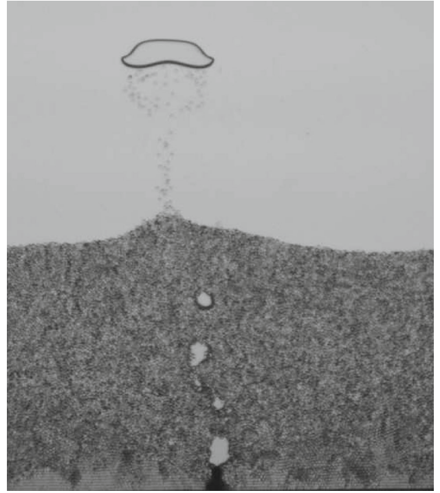
Fig. 10 Bubble carrying on grains in its wake for I = 6.5 mL/min and h_g = 4.5 cm at t = 19.5 s
