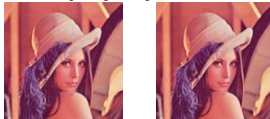
Fig. 13: Left: Reconstructed image by FastNTF-APG with PSNR = 29.00dB (chosen rank R = 20 ), Right: Reconstructed image by FBS4 with PSNR = 29.94dB (chosen rank R = 20 )
