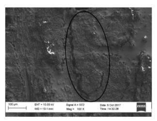
Figure 7. Visualization of wire-matrix decohesion.
