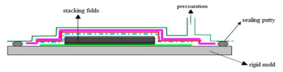
Figure 2. Vacuum molding process.
