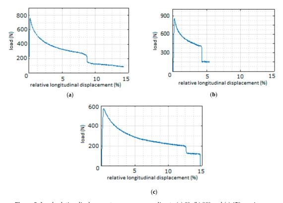
**Figure 5.** Load-relative displacement curve corresponding to (a)  $0^{\circ}$ , (b)  $90^{\circ}$  and (c)  $45^{\circ}$  specimens.
