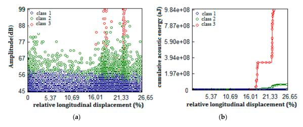
**Figure 14.** (a) Representation of events in amplitude/deformation, (b) cumulative acoustic energy of the different classes for the 45° specimen types.
