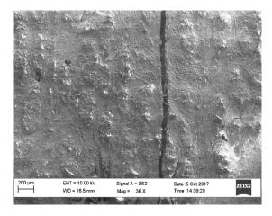
Figure 9. Visualization of delamination.
