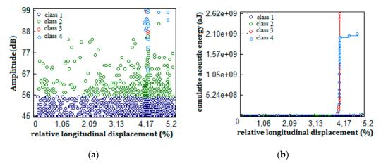
**Figure 13.** (a) Representation of events in amplitude/deformation, (b) cumulative acoustic energy of the different classes for the 90° specimen types.
