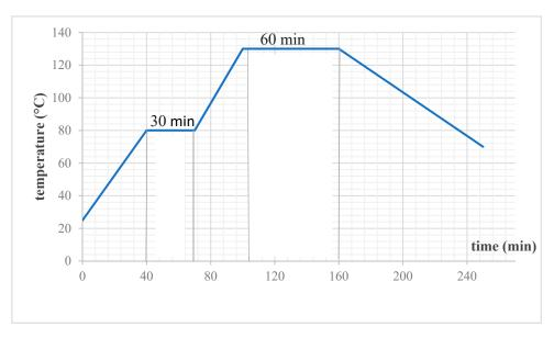
Figure 3. Post-curing cycle.
