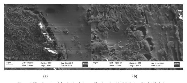
$Figure~8.~\ \ Visualization~of~decohesion~between~fibre/matrix.~(a)~global~view,~(b)~detailed~view.$
