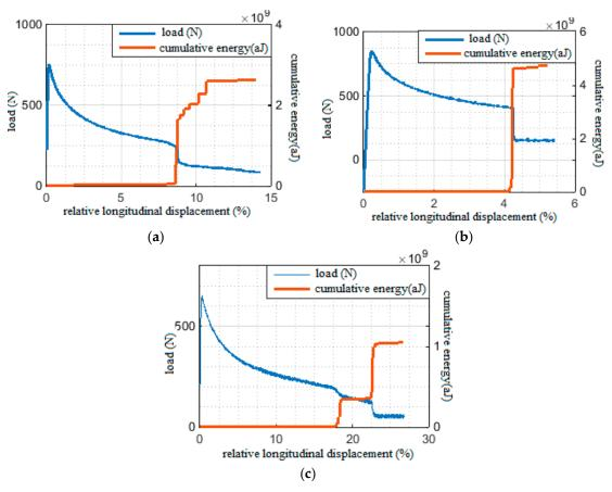
**Figure 15.** Simultaneous evolution of the load and cumulative acoustic energy of (a)  $0^{\circ}$  specimens, (b)  $90^{\circ}$  specimens, (c)  $45^{\circ}$  specimens.
