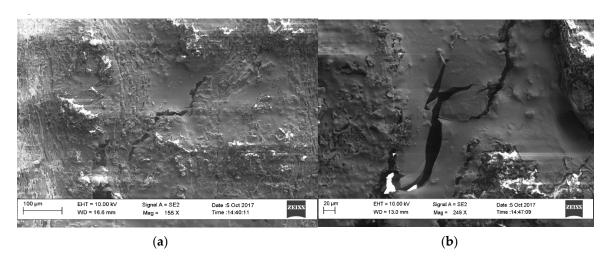
Figure 6. Visualization of matrix cracking. (a) global view, (b) detailed view.
