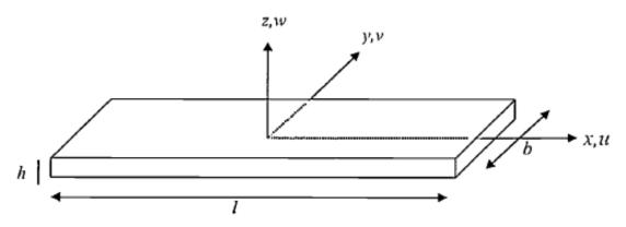
Figure 4. Beam element [21].
