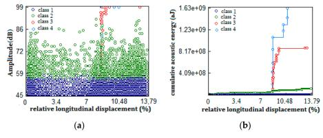
**Figure 12.** (a) Representation of events in amplitude/deformation, (b) cumulative acoustic energy of the different classes for the  $0^{\circ}$  specimen types.
