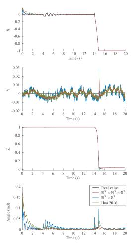
Fig. 4. Plot showing the evolution of estimations from three tilt observers for the simulated biped. The top three figures show each component of the tilt estimation  $\hat{x}_2$  compared to the real value. The bottom shows the error angle for the three estimators.
