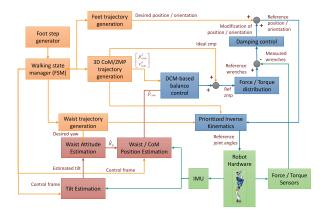
Fig. 5. A simplified diagram of the bipedal locomotion control framework. Elements in red are components related to the estimation. Elements in yellow are components used to generate desired values. Elements in blue are components related to the control. Elements in green belong to the robot.
