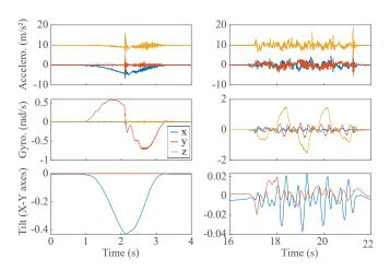
Fig. 7. Plots showing the chest leaning test on the left and the walking test on the right. The accelerometer measurements are on the top, the gyrometer measurements on the middle, and the tilt estimation on the bottom. The Z axis has been removed from the tilt estimation for legibility and can be reconstructed knowing that it is the positive solution to the vector normality constraint.
