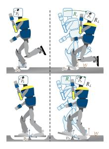
Fig. 1. Model of the anchor point definition in the case of non fixed anchor. In the top an example of single support phase and in the bottom a double support. The origin of the control frame  $\mathcal C$  is located at the position of the anchor point. The origin of the world frame  $\mathcal W$  can be located anywhere. The rotation  $R_{\mathcal C}$  between the world frame  $\mathcal W$  and the control frame  $\mathcal C$  is not available with encoders.
