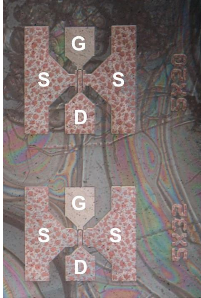
FIG. 2. Backside optical view (50 x) of HEMTs with low cracks in GaN layer after Si substrate removal.
