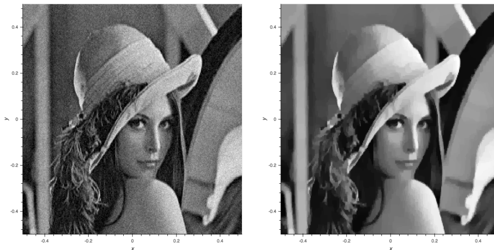
Figure 4: Example of TV Denoising with model (58)
