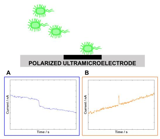
**Figure 1.** Schematic representation and typical electrochemical signal for single nano-impact experiments of *Shewanella oneidensis* bacteria recorded at a 7  $\mu$ m carbon ultramicroelectrode polarized at (**A**) +0.6 V *vs.* Ag/AgCl in 20 mM potassium ferrocyanide and (**B**) -0.3 V *vs.* Ag/AgCl in 20 mM potassium ferricyanide with 20 mM potassium phosphate buffer at pH 7.2 as aqueous electrolyte.
