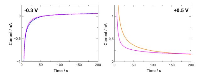
**Figure S3.** Chronoamperometric measurements recorded at two different potentials (*vs.* Ag/AgCl) at a 7  $\mu$ m carbon ultramicroelectrode in 20 mM potassium phosphate buffer at pH 7.2 as aqueous electrolyte (pink curves) with 20 mM K<sub>4</sub>Fe(CN)<sub>6</sub> (blue curve) and K<sub>3</sub>Fe(CN)<sub>6</sub> (orange curve) under inert atmosphere (Ar) in the presence of *Shewanella oneidensis* bacteria in solution.
