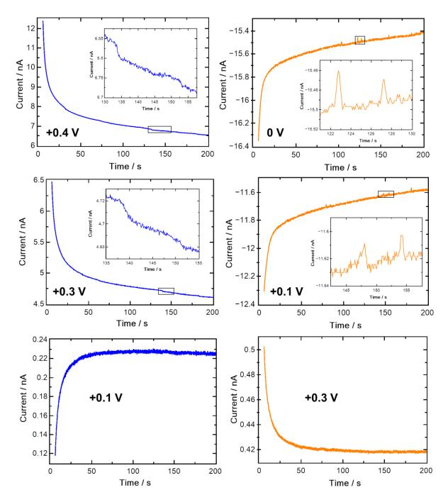
**Figure S2.** Chronoamperometric measurements recorded at different potentials (*vs.* Ag/AgCl) at a 7  $\mu$ m carbon ultramicroelectrode in 20 mM K<sub>4</sub>Fe(CN)<sub>6</sub> (LEFT, blue curves) and K<sub>3</sub>Fe(CN)<sub>6</sub> (RIGHT, orange curves) in 20 mM potassium phosphate buffer at pH 7.2 as aqueous electrolyte under inert atmosphere (Ar) in the presence of *Shewanella oneidensis* bacteria in solution.
