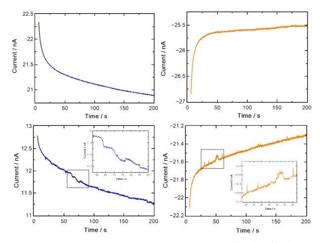
**Figure 2.** Chronoamperometric measurements recorded on 7  $\mu$ m carbon ultramicroelectrode at +0.6 V *vs.* Ag/AgCl in 20 mM K<sub>4</sub>Fe(CN)<sub>6</sub> (LEFT, blue curves) and -0.3 V *vs.* Ag/AgCl in 20 mM K<sub>3</sub>Fe(CN)<sub>6</sub> (RIGHT, orange curves) in 20 mM potassium phosphate buffer at pH 7.2 as aqueous electrolyte under inert atmosphere (Ar) in (TOP) the absence and (BOTTOM) the presence of *Shewanella oneidensis* bacteria in solution.
