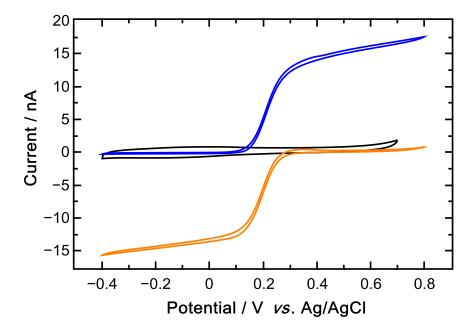
**Figure S1.** Cyclic voltammograms recorded at 20 mVs<sup>-1</sup> at a 7  $\mu$ m carbon ultramicroelectrode in 20 mM potassium phosphate buffer at pH 7.2 as aqueous electrolyte (black) with 20 mM K<sub>4</sub>Fe(CN)<sub>6</sub> (blue) and K<sub>3</sub>Fe(CN)<sub>6</sub> (orange) under inert atmosphere (Ar).
