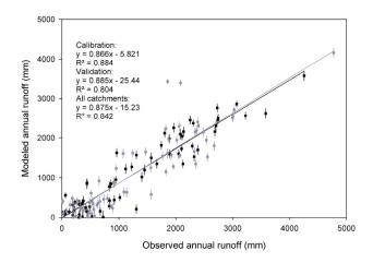
**Fig. 3.** Observed versus modelled annual runoff of catchments used for calibration (N=69, black dots), validation (N=69, gray dots), and all (N=138). Each dot represents observed average annual runoff for one catchment. The error bar represents the effect on modelled runoff of a  $\pm 10\%$  change in catchment evapotranspiration to account for the mismatch between current and potential vegetation cover simulated by MAPSS.
