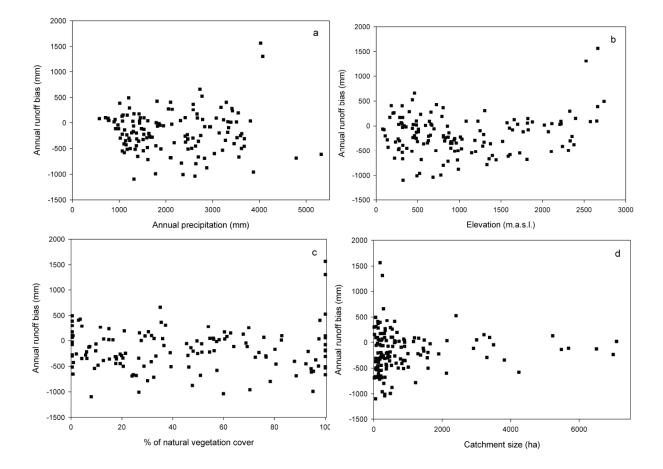
**Fig. 5.** Residual distributions of annual runoff according to catchment annual precipitation (**a**), average elevation (**b**), percentage of natural vegetation cover (**c**), and size (**d**). Each dot corresponds to the difference between MAPSS-modelled and observed annual runoff for each catchment.
