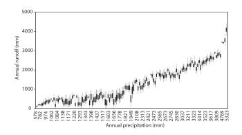
**Fig. 6.** MAPSS model runoff uncertainty obtained by a Monte Carlo-type approach (Latin Hypercube Sampling). For each catchment, the black line shows the whole range of predicted values and the box ranges within one standard deviation from the mean. Catchments were ordered according to annual precipitation. (Horizontal axis does not show all catchment values).
