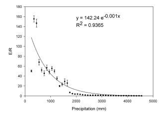
**Fig. 10.** Modelled evapotranspiration-runoff ratio (E/R) along the annual precipitation gradient across the Mesoamerican region. Each point represents a 100 mm annual precipitation class. Bars show standard error of each class.
