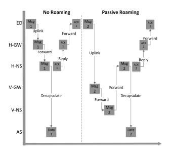
Fig. 10. Communication Mechanism in Passive Roaming
