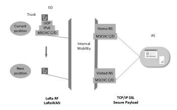
Fig. 12. Deploying of MSCHC mechanism on LoRaWAN Architecture
