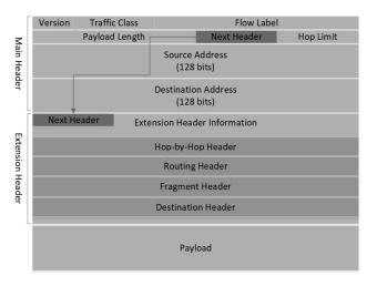
Fig. 4. MIPv6 main Header and Extension Fields
