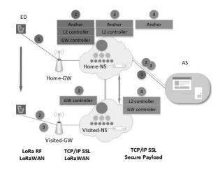
Fig. 9. Types of Roaming supported in LoRaWAN.
