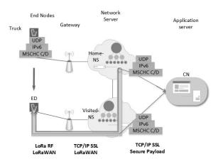
Fig. 16. Tunneling with CN using routing optimization
