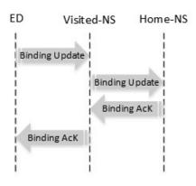
Fig. 14. Registration mechanism
