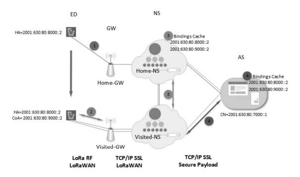
Fig. 17. Handover Procedure in LoRaWAN using MIPv6 compressed by MSCHC
