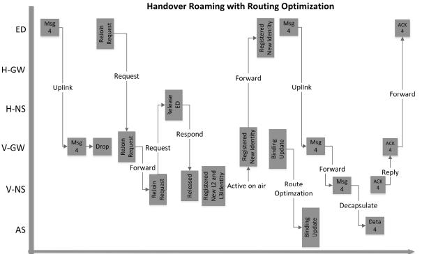
Fig. 11. Communication Mechanism of ED in Handover Roaming
