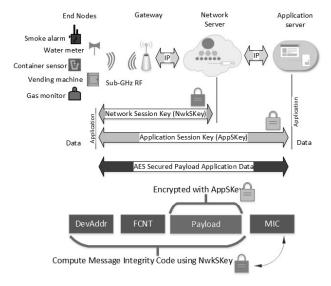
Fig. 5. LoRaWAN Architecture
