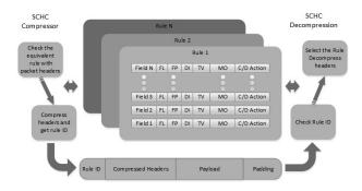
Fig. 2. SCHC Standard Implementation Architecture
