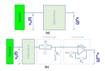
FIGURE 5. Diagram of (a) distorted and (a) reconstructed sensor with NGD circuit topology.
