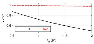
FIGURE 13. Comparison of cross correlations between the distorted ("black solid line") vs reconstructed ("red dashed line") and sensored signals.
