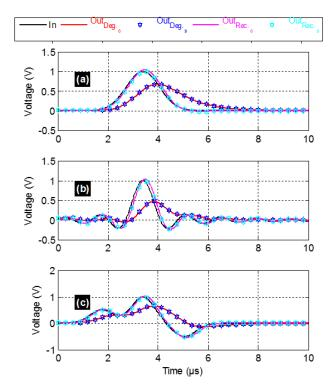
FIGURE 14. Comparison of simulated and calculated transient responses form the NGD reconstructed circuit shown in Fig. 6: (a) Gaussian, (b) sinc and (b) arbitrary waveform pulse signals.
