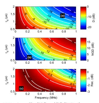
**FIGURE 7.** Cartographies of (a) distorted ("D"), (b) NGD and (c) reconstructed ("Rec.") calculated TF magnitudes versus  $\tau_d$  and frequency.
