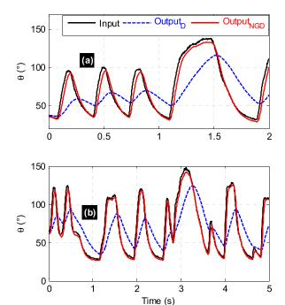
FIGURE 17. Comparison of distorted and reconstructed measured transient signals form the experimental setup shown in Fig. 15 with: (a) 2 s and (b) 5 s time durations.
