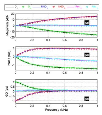
FIGURE 11. Comparison of simulated and calculated TF (a) magnitudes, (b) phases and (c) GDs of the reconstructed circuit POC shown in Fig. 6.
