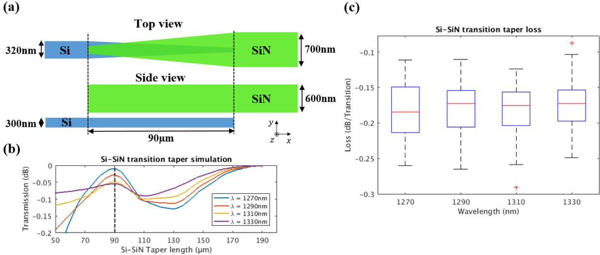
Figure 5. Development of an adiabatic Si-SiN transition taper. (a) Schematic view of the transition taper. (b) Numerical simulation (EME solver<sup>22</sup>) of the taper length impact on transmission performance. (c) Statistical measurement of Si-SiN 90 $\mu$ m transition loss (30 die, 1 wafer).
