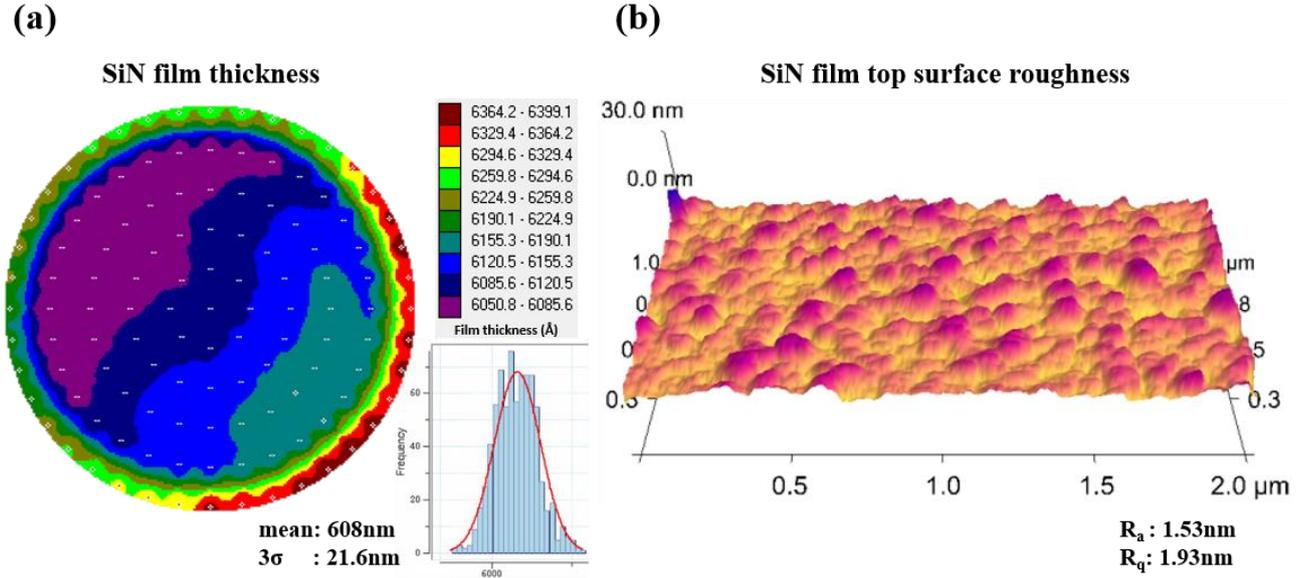
Figure 2. Analysis of the SiN film properties on a 300mm wafer. (a) Ellipsometric measurement of SiN film thickness uniformity (128 points, 1 wafer). (b) AFM picture of SiN film top surface ( $2 \times 1 \mu\text{m}$  window, wafer center).  $R_a$ : arithmetic average of surface height deviation.  $R_q$ : root mean square average of height deviation.
