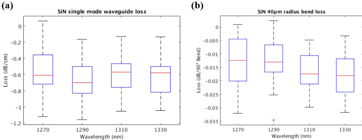
Figure 4. Statistical measurements of SiN waveguide and bend. (a) Single mode TE-polarization SiN waveguide propagation loss (30 die, 1 wafer). (b) SiN 40 $\mu$ m radius TE-polarization bending loss (30 die, 1 wafer).
