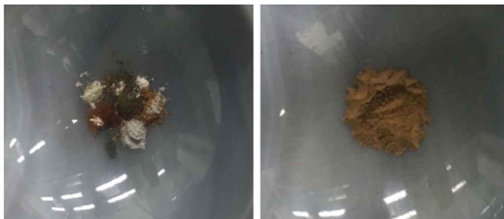
Figure 2. The 14 individual mineral phases weighed out in the mortar (A) before mixing and (B) mixed together.
