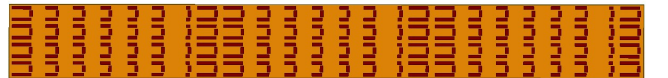
Fig. 3. Metasurface design using the optimized dimensions of 4 \times 3 super-cells, of dimensions 25\text{ mm} \times 215\text{ mm} , with a ground plane and substrate of permittivity \epsilon_r = 2.2 and thickness 1.6 mm.
