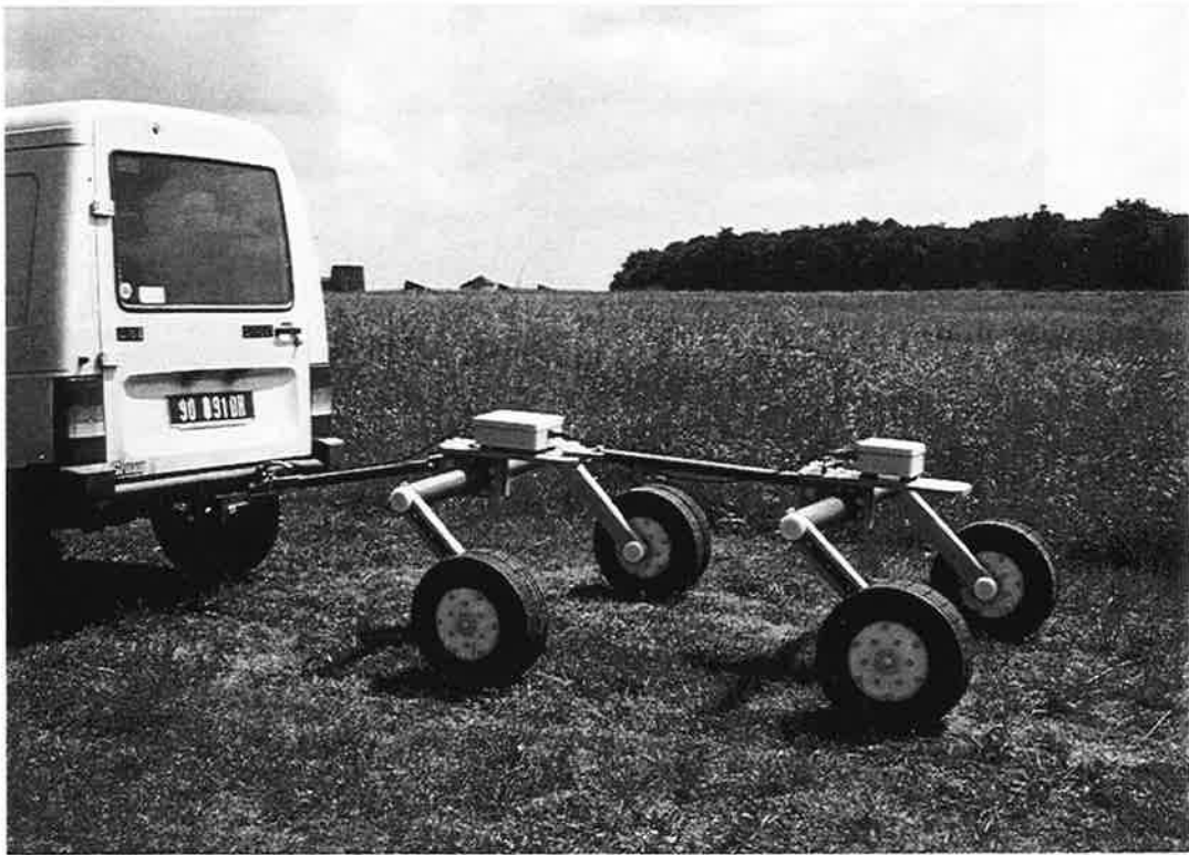
Fig. 5: The new electrostatic quadrupole: the electrodes are contained in the wheels.
