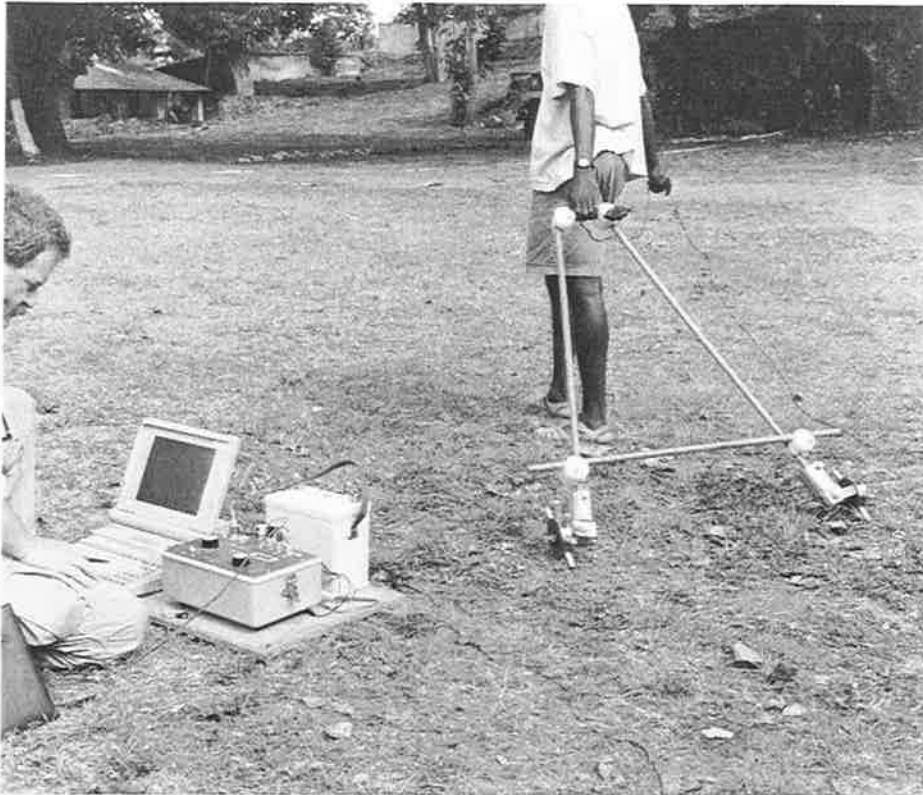
Fig. 3: Experimental prototype of a «twin electrodes» array for resistivity recording with the RATEAU acquisition system.
